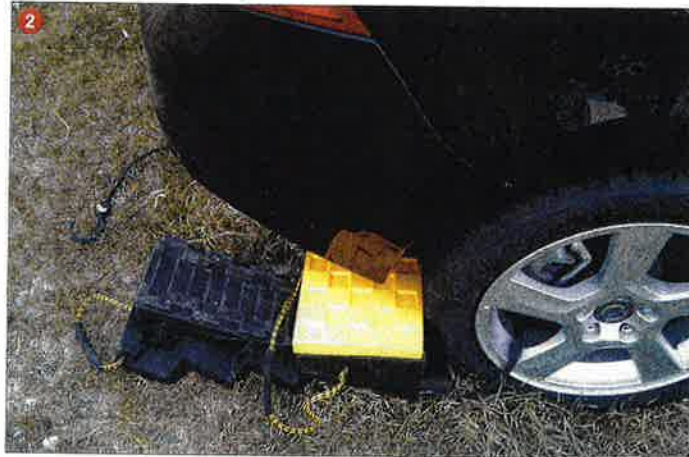
(2) The user positions the Cog Step as needed, with the cog wedge in close proximity to where it is needed to effect stabilization. As rescuers unweight the side of the vehicle, as they would to place a standard step chock, they introduce the Cog Step in much the same way. (Photo by author.)
